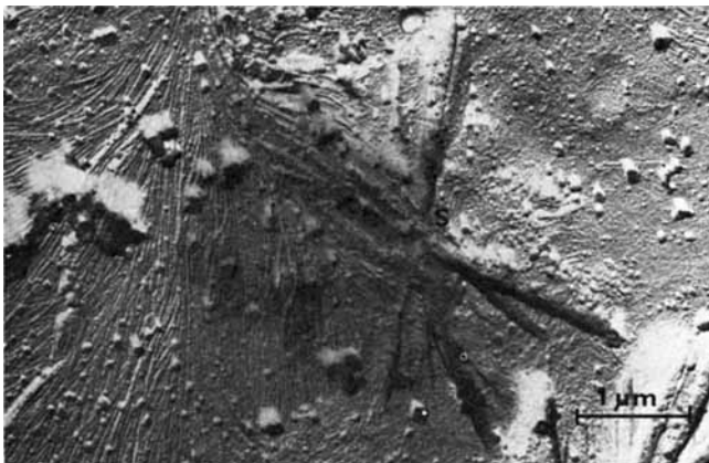
Fig. 12. Morphology of the PP-Q sample etched 5 min at 25°C in 5% Mn-S mixture. \text{MnO}_2 precipitated on the surface was not dissolved and forms a grainy structure. S marks a large star-shaped artefact.
